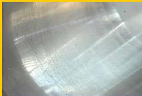
In all the liners you could see distinct traces of the cross-honing pattern of the original bore, and the liner surfaces looked "polished-like" and shiny like in a new engine.
